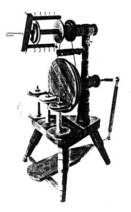
If there is too much tension on the brake band, the yarn will pull in too quickly or break.
